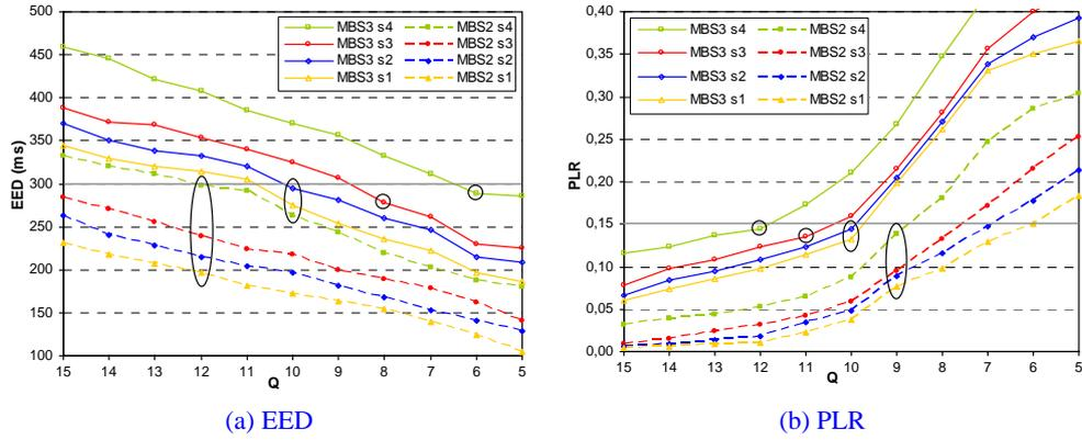
Fig.5 EED and PLR depending on Q, for different MBS and s combinations (RT.Audio).
