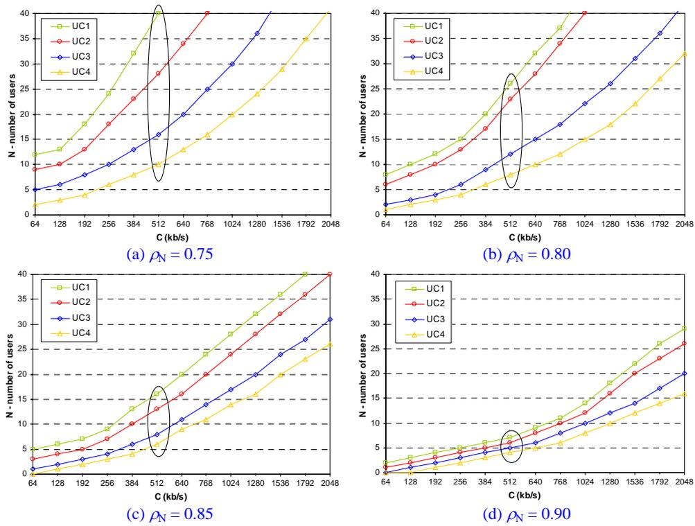
Fig. 7. Recommended performance areas for the variation range of capacity ( $C$ ) and number of users ( $N$ ), depending on the useful thresholds and relative link occupancy factor ( $\rho_N$ ).
