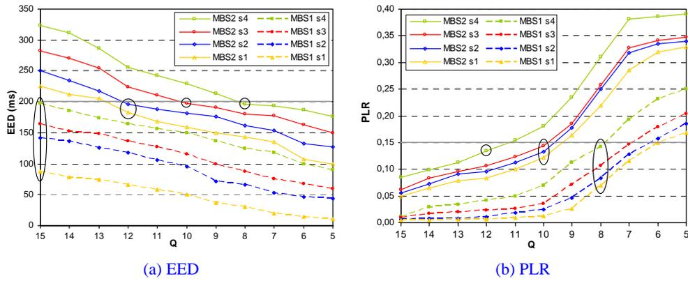
Fig.6 EED and PLR depending on Q, for different MBS and s combinations (RT.Video)
